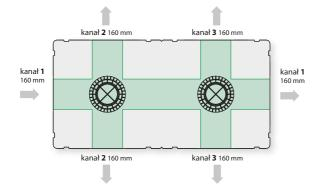
openings 200 mm in diameter provide access from the ground all the way to the bottom of the tank for purposes of inspection and cleaning. There are 6 openings 160 mm in diameter in the side walls and 2 openings 200 mm in diameter at the top of the box. Supply pipes 200÷500 mm in diameter can be connected to the side of Stormbox using an adaptor.
