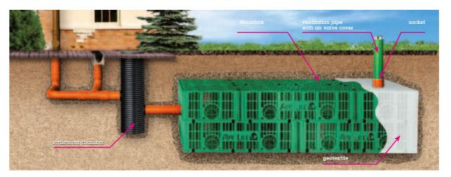
Diagram showing the Stormbox rainwater infiltration system
