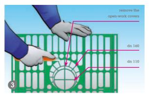
All the open-work covers should be removed at the expected locations of inspection manholes or vertical riser pipes (both along the horizontal and the vertical channels).
