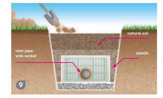
9. Fill the sides with 15 - 30 cm layers of gravel pack, grain size e.g. 8 - 16, 12 - 24 (30) mm, or with coarse sand. Even out and compact the ground. Adjust the ground compaction level to the expected loads.
