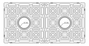
the boxes and cutting out a hole matching the diameter of the pipe, insert a PVC-U, PP-B pipe approx. 20 cm long. Carefully secure the connection so as to prevent the soil from entering the box module.
