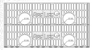
In order to connect the plain ends of PVC-U, PP-B  $d_n$  110, 160 mm pipes to the side walls, cut out the polypropylene reinforcements from the inlet openings. After wrapping geotextile around
