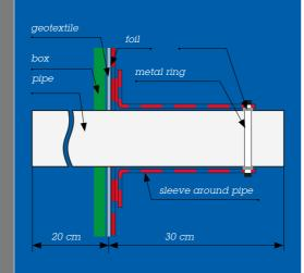
Diagram showing the method of sealing a pipe opening in the wall of the box.
